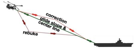
As the helicopter approached the ship, the radar operator would direct the pilot to maintain 500 feet of altitude until he intercepted the glide slope.
