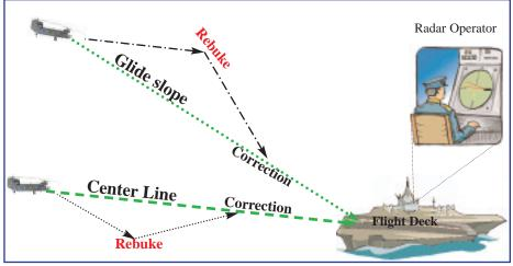
If the radar return confirmed that the pilot was on both lines, the operator would continue to report, "On course, on glide slope." If everything went perfectly, those were the words the pilot would hear until he landed on the flight deck.
